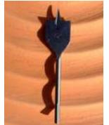
To fill the water butt with the recommended 3P Filter Collector Universal, select the 32 mm flat bit from the set provided with the filter.
