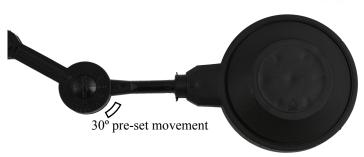
This is the pre-set articulation point that allows the tank level to decrease, without opening the regulator. This works because the arm allows the float to move before the arm engages with the regulator.
