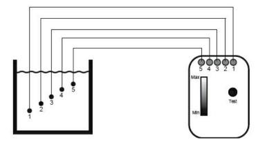
The maximum cable length for the Indicator to function is 30m. The individual cores of the cable are cut to length dependant on the tank depth. (see illustration)
