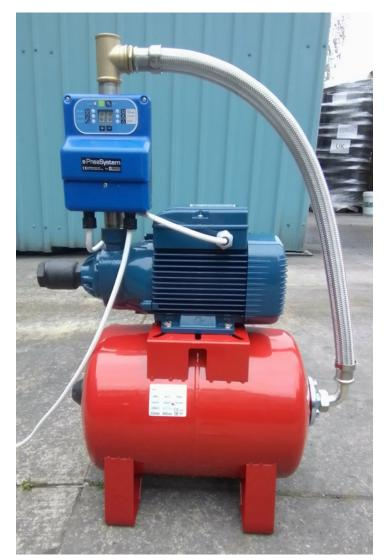
Failure or discharged status of the pressure vessel is immediately detected and the pump shut down to prevent damage. Dry run protection is by pressure loss and CosPhi monitoring, and dry running can be further prevented by the optional use of a float switch.
