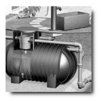
Installation in soakaway shaft or infiltration system
