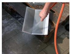
Check to see if water passes easily through the sieve, if so reinsert it and screw into position.
