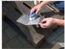
Also clean the back surface, brushing in horizontal and vertical direction, before finally rinsing with a water spray action.
