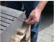
Withdraw the filet mesh sieve plate
