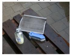
Wet the sieve, spray some cleaning liquid on it, and then brush in both horizontal and vertical directions.
